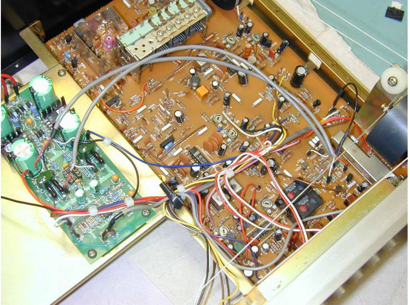
Figure 12, Wiring from Tuner Main Board to TM-1001 Power Supply and Amplifier Board
