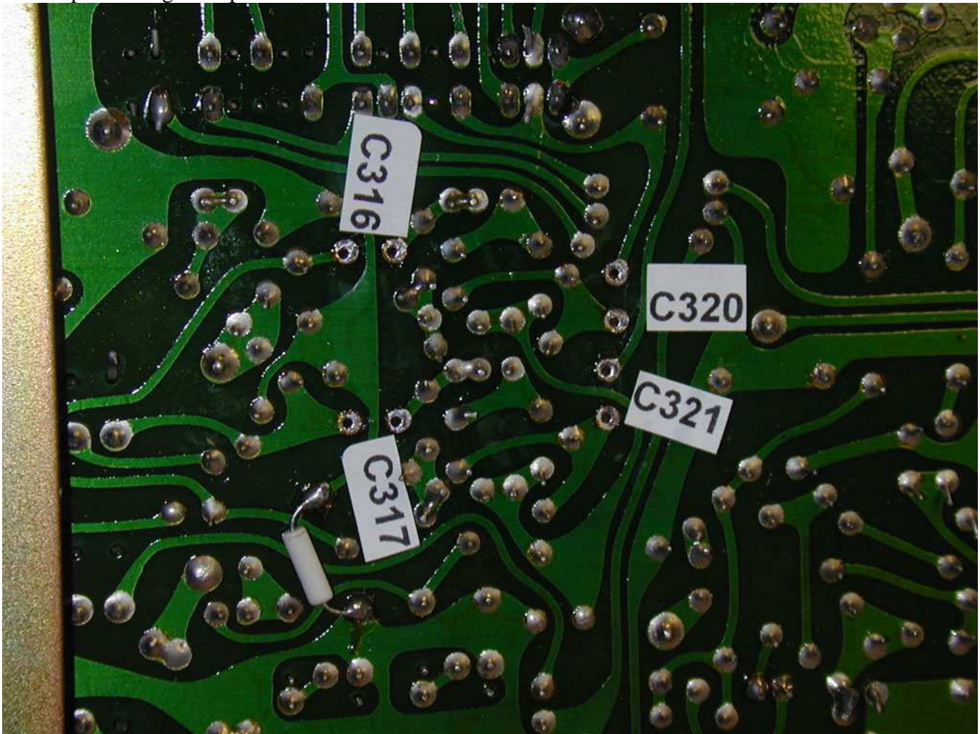
Figure 9, Capacitor locations on underside of main board
