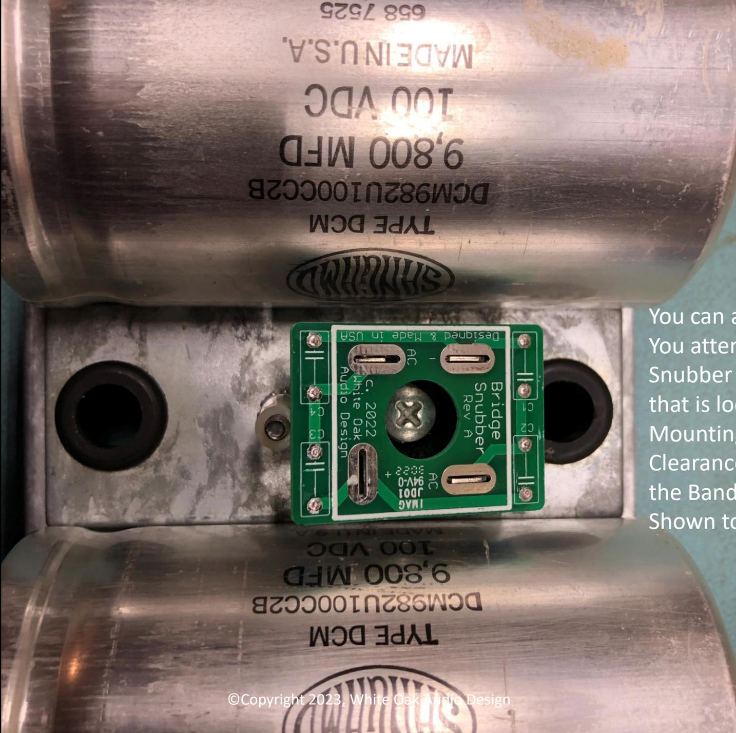
You can also observe that when you attempt to install the bridge snubber board on the bridge that is located in the original rear mounting hole position that a clearance problem is created with the band clamp mounting screw shown to the left.
