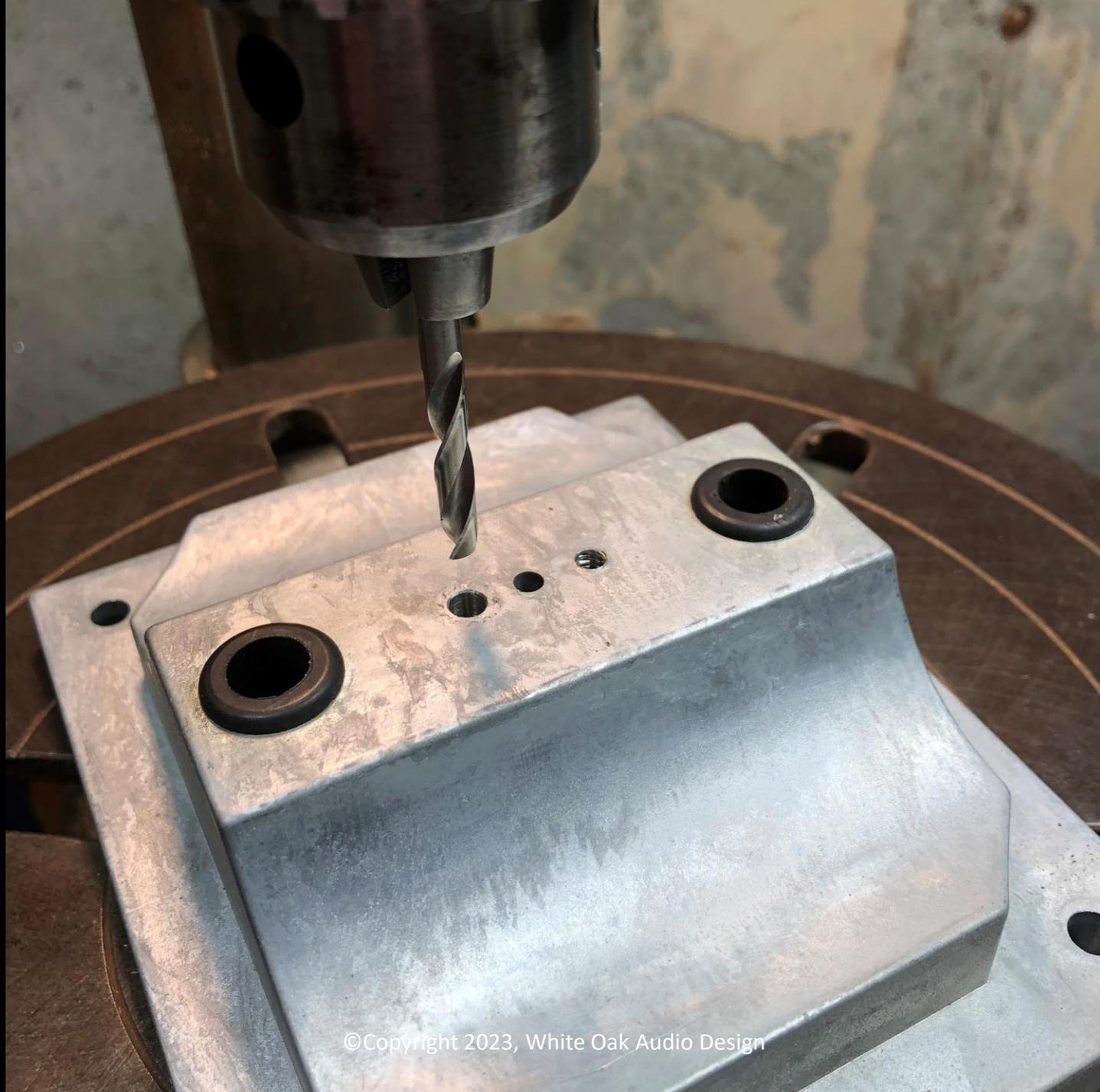
This is the location to Bore out. The location With the enlarged die Cast boss seen on the bottom Side of the transformer Cradle.
