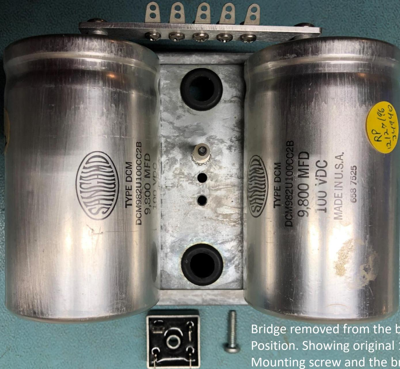
Bridge removed from the bottom hole Position. Showing original 10-24 self-tapping Mounting screw and the bridge rectifier
